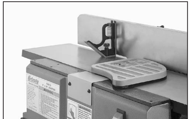
Figure 27. Checking the 90° stop.
